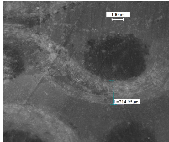
Fig. 14. Cross section of a weft yarn
