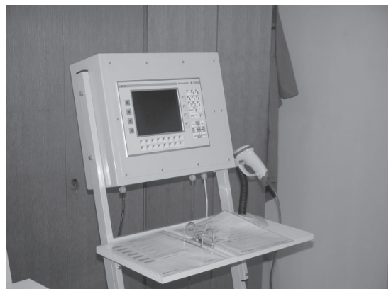
Fig. 1. A terminal used to record production events (manufactured by Kolektor Sinabit Ltd.)
