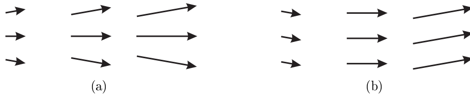
Figure 5.1 The (a) length-splay and (b) length-bend distortions, accounted for by the L_6 and L_7 terms, respectively.
