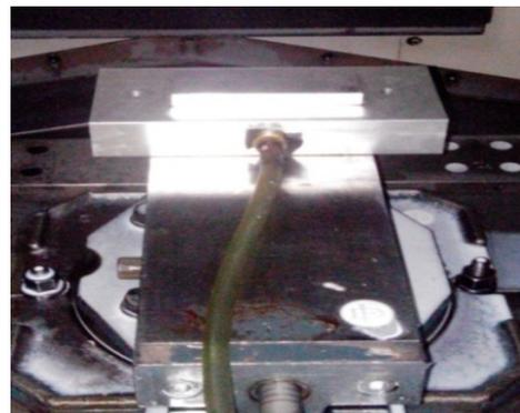
**Fig. 3** Work piece held on vacuum fixture
