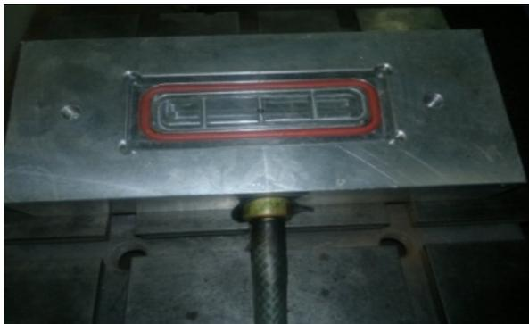
**Fig. 2** Shop made vacuum fixture used for experiments [19]
