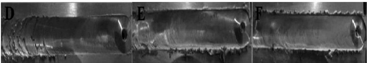
Figure 5: Photograph of samples processed at a rotational speed of 1600 \text{ min}^{-1} and travel rates of: d) 100 mm/min, e) 200 mm/min and f) 300 mm/min
