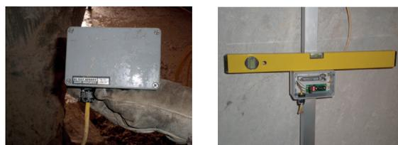
**Figure 6:** Vertical EL beam gauge installation on the high safety pillar VS3.
