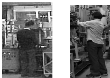
Fig. 8 A typical photograph of piston rod circlipping event at traditional and semi-ergonomic shocker assembly line
