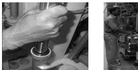
Fig. 10 A typical photograph of oil seal pressing event at traditional and semi-ergonomic shocker assembly line
