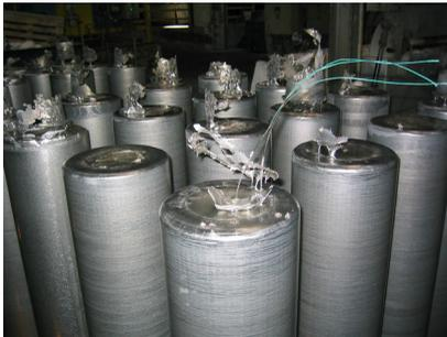
Fig. 6. Billet instrumented with thermocouples for temperature measurement
