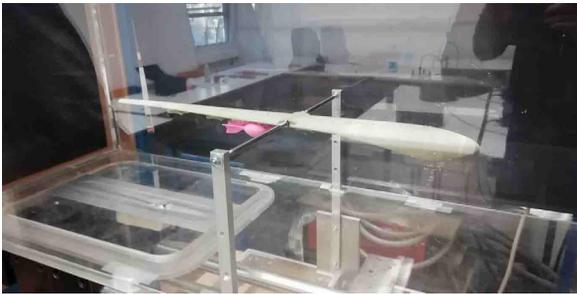
Fig. 23. Fuselage drag measurement in wind channel
