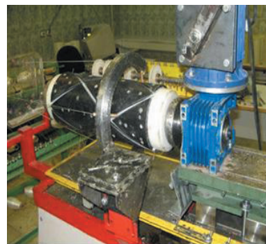
Fig. 1. Specimen fabrication using a filament winding process [4]
