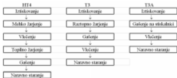
Slika 1: Sheme postopkov za toplotno obdelavo zlitine AlCuMgPb Figure 1: Schemes of heat treatment of AlCuMgPb (AA2030) alloy
