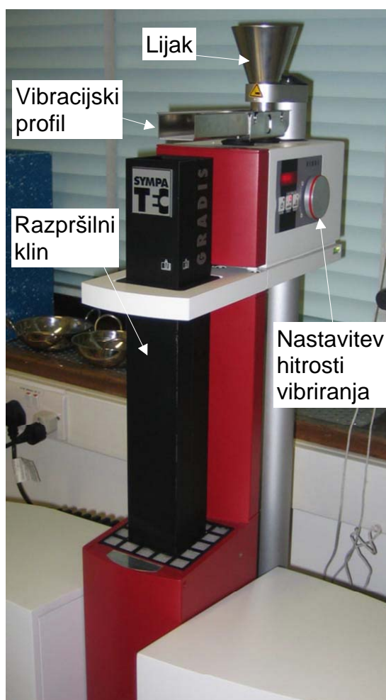
Slika 3.46: Nastavek GRADIS za suho analizo geometrijskih lastnosti zrn Figure 3.46: GRADIS adapter for the dry analysis of the geometrical properties of particles
