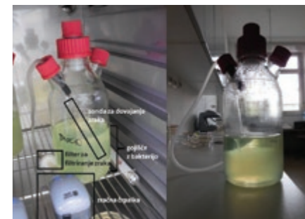
Slika 2: B_0 (levo), posedena biomasa v B_0 ob koncu eksperimenta (desno) Figure 2: B_0 (left), settled biomass in B_0 at the end of the experiment (right)
