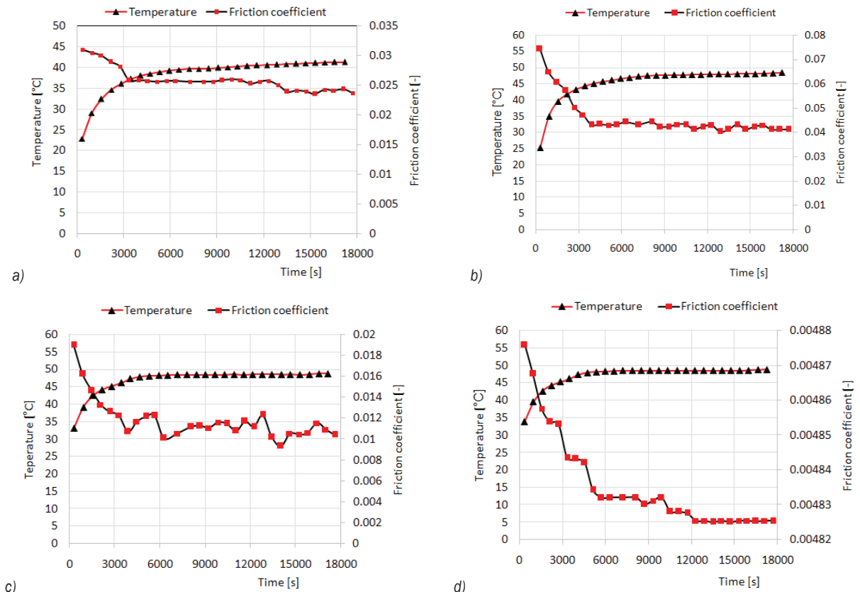
Fig. 5. Trends in time of friction coefficient and bearing temperature at 1000 rpm speed, for a load of a) F_N = 1000 N; b) F_N = 2000 N; c) F_N = 3000 N and d) F_N = 4000 N
