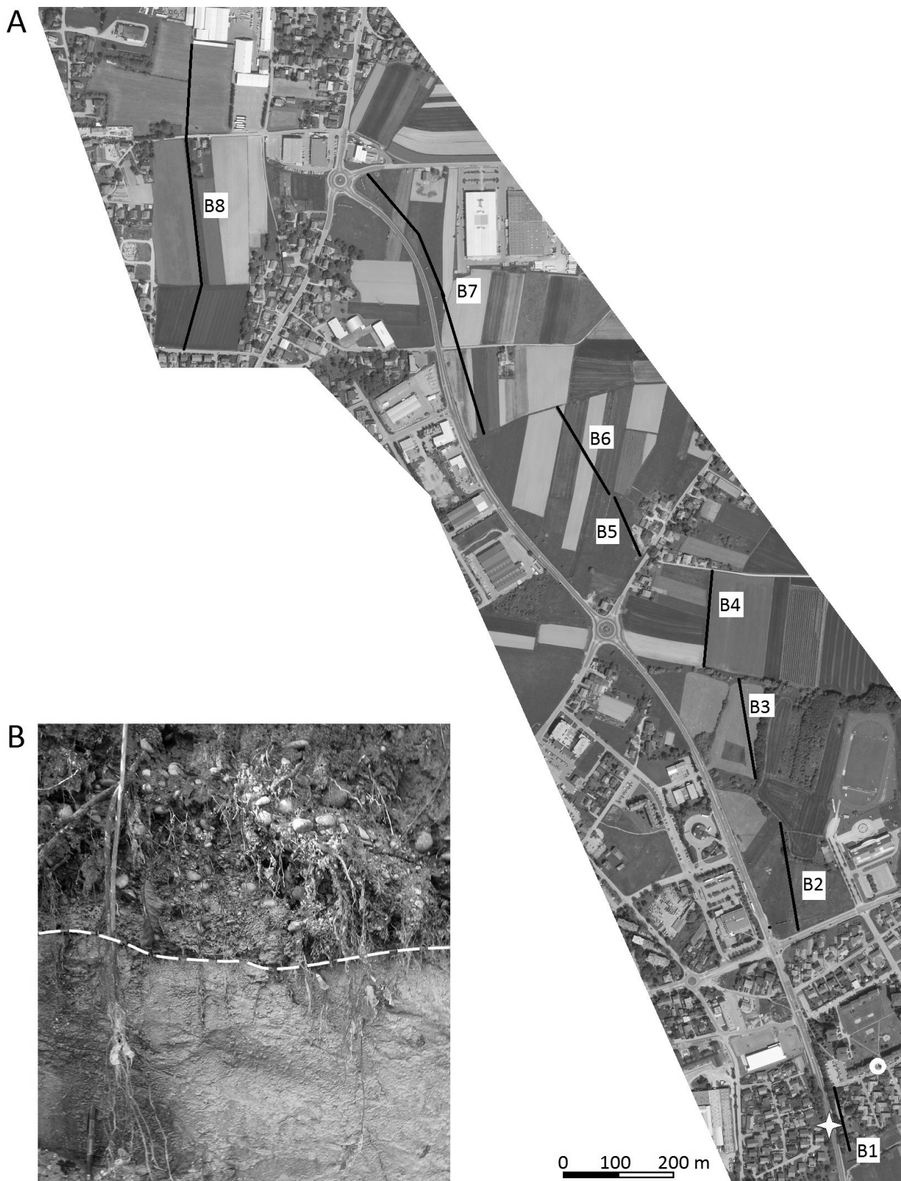
Fig. 3. A – Position map of GPR profiles B1 to B8 recorded across the BSRT (lines), location of borehole used for depth calibration (circle east of B1) and location of outcrop image in B (star W of B1); B – Erosional contact (dashed line) between Pannonian marl and overlying Quaternary sediments of the BSRT in the newly-opened road cut through the BSRT.
