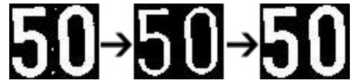
Figure 2: On the left we have the original segmented image. We then perform two morphological operations - first erosion (middle image) and then dilation (right image). The result is the symbol with the original size but without the noise.
