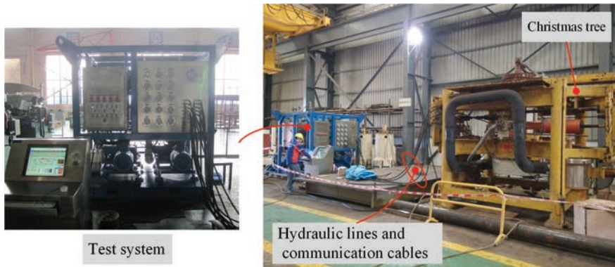
Fig. 3. Subsea Christmas tree testing system
