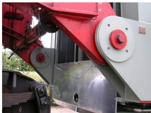
Figure 2: Connection between the transformer and the Schnabel wagon
