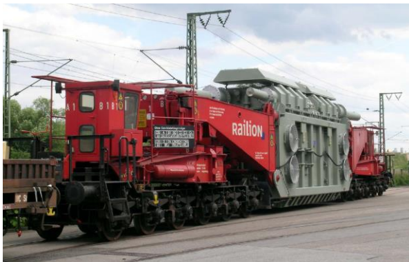
Figure 3: Schnabel wagon with a cage-tank acting as a “bridge”
