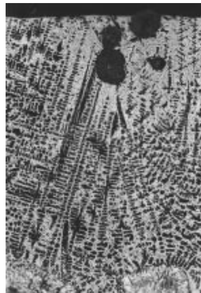
Slika 2: Mikrostrukturni posnetek pretaljene cone, pove-ava 500x Figure 2: Microstructure of the remelted zone, 500x
