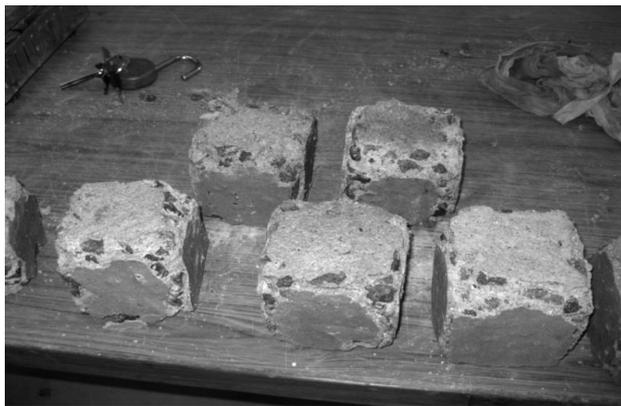
**Figure 1:** GPC samples after 180 d in sulphuric acid
