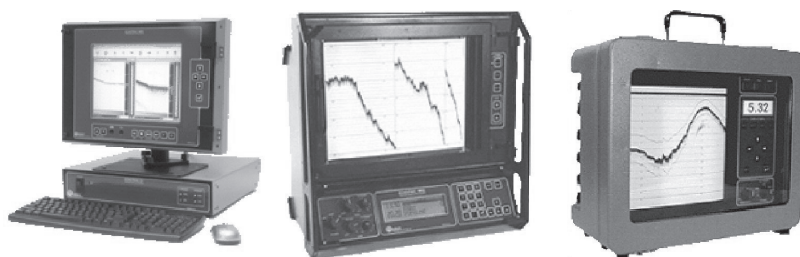
Slika 2: Primeri singlebeam globinomerov proizvajalca Odom: Echotrac CV, Echotrac MKIII, Hydrotrac ( www.odomhydrographic.com ).
