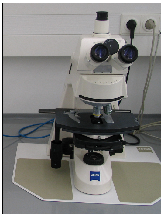
Figure 7: Example of a reflected light microscope. Note that the objectives are above the specimen table and light comes from above the specimen table.
