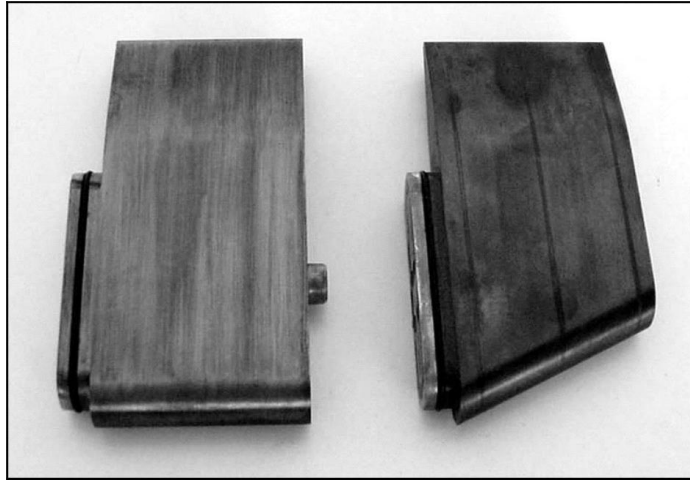
Sl. 1. Osnovni profil – PPVR (levo) in spremenjeni – PNVR (desno) Fig. 1. Basic – CLE (left) and modified – ALE hydrofoil (right)
