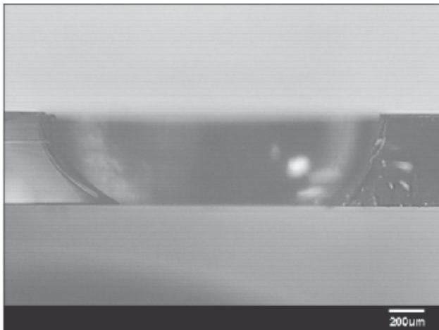
Fig. 4: Cross-section view of the through-etched hole with a Cr/Au photoresist mask for an annealed glass.
