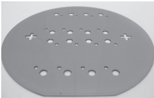
Fig. 5: 500µm-thick Pyrex glass wafer etch-through using a:Si/SiC/ PR mask (the mask was kept on the wafer)
