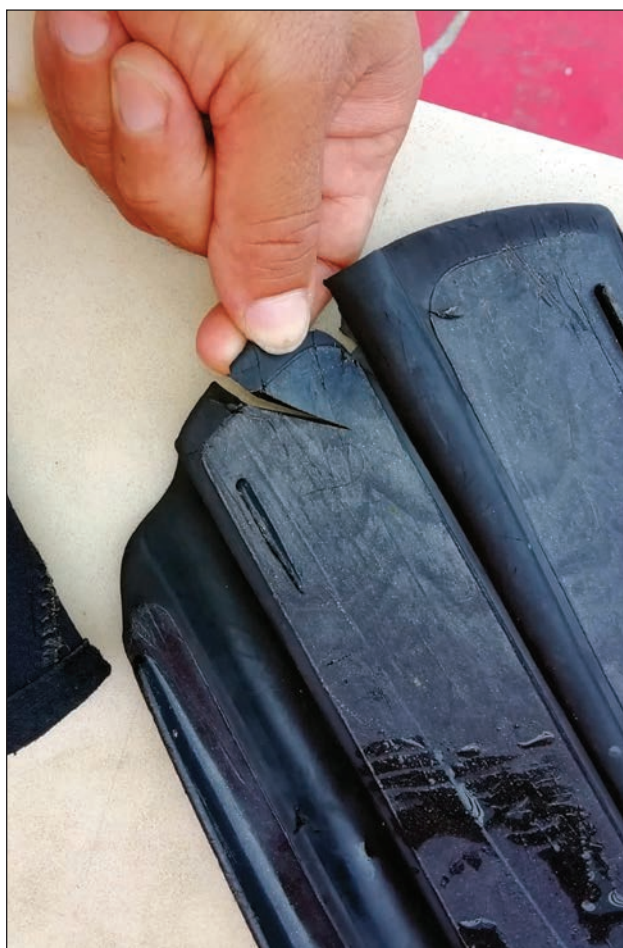
Fig. 3: Lacerations on fin belonging to diver 1 (Photo: İbrahim Yörüsün).
