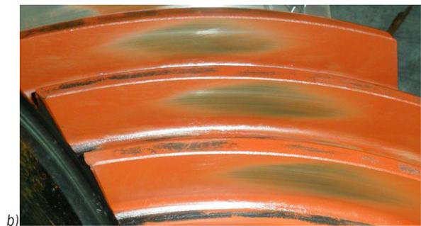
Fig. 10. Tooth bearings on the hypoid gear test machine for the hypoid gear drive 7×43; a) drive side, and b) coast side
