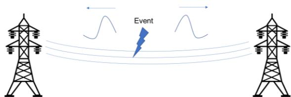
Figure 1: Representation of traveling-wave on power cables
