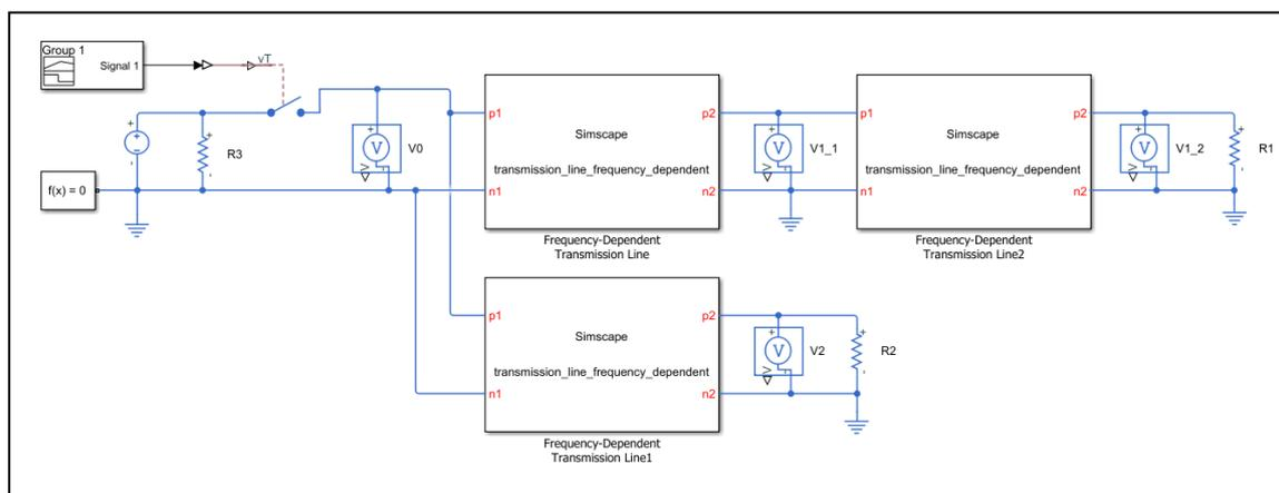
Figure 2: Simulation power cable model
