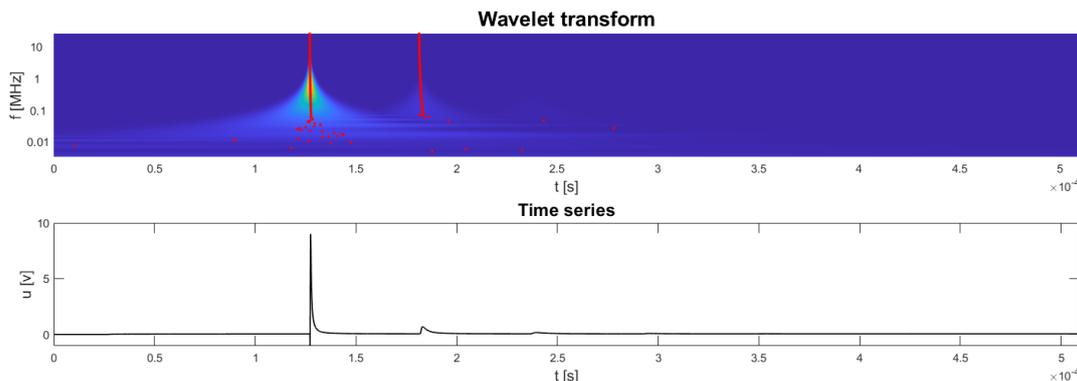
Figure 4: Time-series signal and signal wavelet transform at cable end V2.
