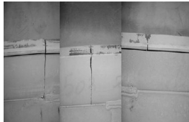
Figure 7: Cracks in the central stiffener, both sides and the lateral stiffener (after panel dismantling) Slika 7: Razpok v centralnem rebri, obe strani in bočna utrditev (po demontaži panela)
