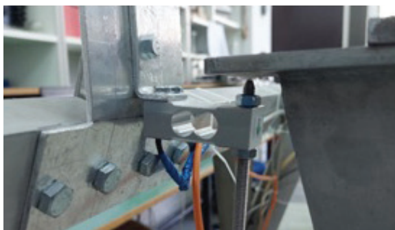
Fig. 2. Load cell for thrust force measurement
