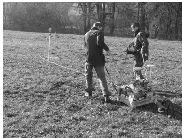
Fig. 3. Ground Penetrating Radar (GPR), the position of which is recorded by the proposed hybrid positioning system, comprising a GPS receiver SR 20, georeferenced by GS 20 (Leica), and the dead reckoning (DR) accelerometer subsystem, in use at an archeological site. Both positioning devices are placed at the top of the GPR antenna.
