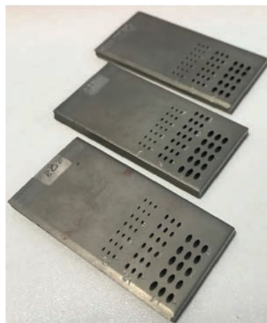
Fig. 7. Inconel 718 test samples
