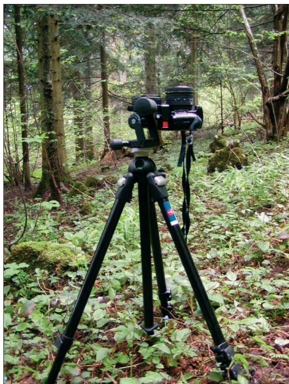
Figure 2: Sigma 8mm fisheye lens mounted on Nikon F601 camera body on the tripod with levelling head that ensures horizontal position of the lens.
