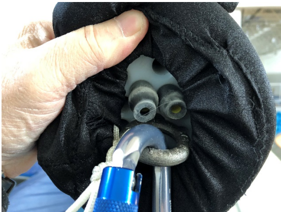
Figure 2. Attachment of bungee cords.
