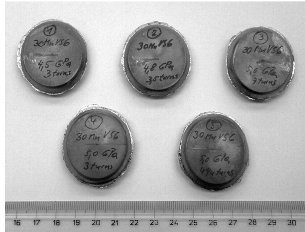
Figure 3: Final products of the HPT process Slika 3: Končni proizvod HPT-postopka
