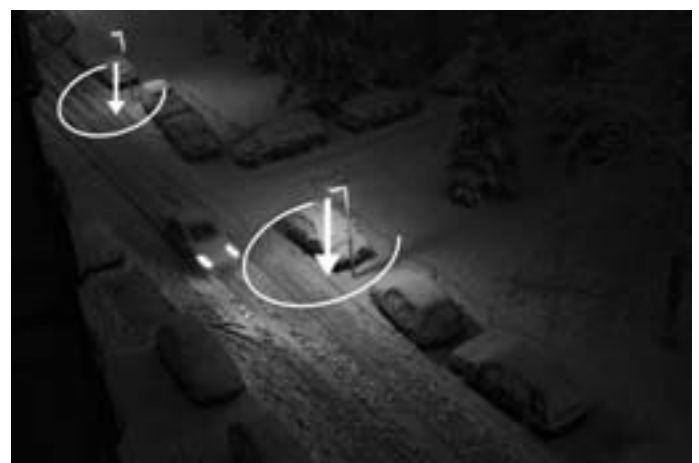
Slika 10: Nezasenčene in usmerjene svetilke. Un-shaded and directed lighting.
