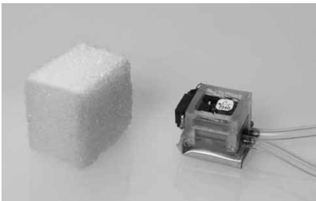
Fig. 3: Pump cube compared to a sugar cube. The system comprise a silicon micro pump chip, driver electronics together with micro controller, silicone gasket, fluidic carrier, and battery. The Pump cube is the smallest pump system worldwide.
