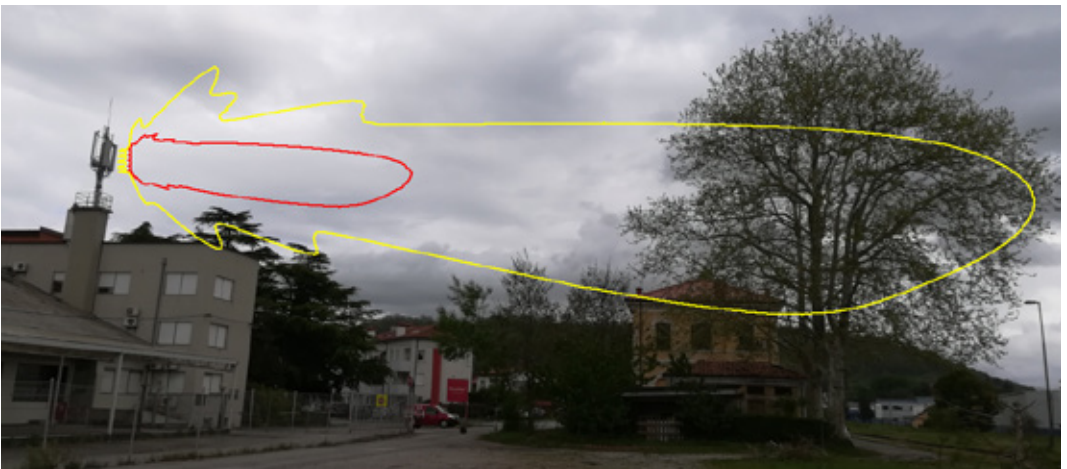
Figure 3.6: Compliance zone for a typical 3G – 5G base station according to Slovenian legislation: yellow for I. area of protection, red, for II. area of protection. Limit values for II. area of protection is similar to ICNIRP guidelines and 1999/519/EC recommendation, for the I. area of protection, the limit values are 10 times lower (for power density).
