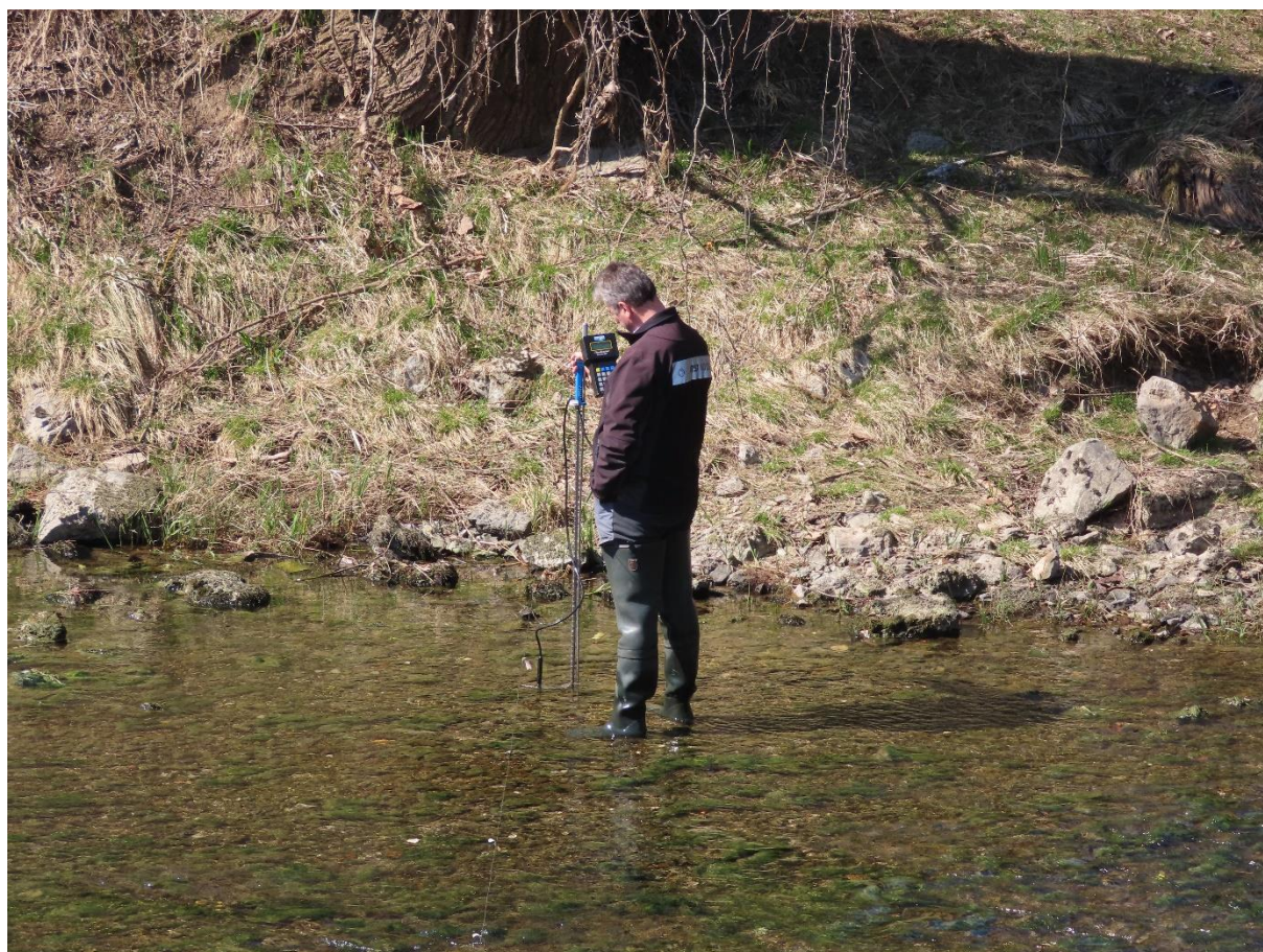
Slika 6. Izvajanje meritve pretoka ob nizkem vodnem stanju marca 2022 (foto: Arhiv ARSO) Figure 6. Discharge measurement during low water conditions in March 2022 (Photo: ARSO Archive)
