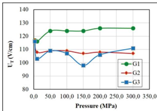
**Figure 6:** Threshold voltage  $U_T$  (V/mm) of the varistor ceramics from granulates G1, G2 and G3, uniaxially pressed at different pressures and sintered at 1200 °C for 2 hours.
