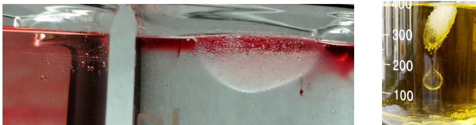
Figure 1.3. On the left, surfaces of the experiment described in the text with the ice (on the left in pure water and on the right in water saturated with salt); it can be observed the formation of condensation water droplets, on the outside of glass cans, in the second case. On the right, ice in cooking oil at room temperature.
