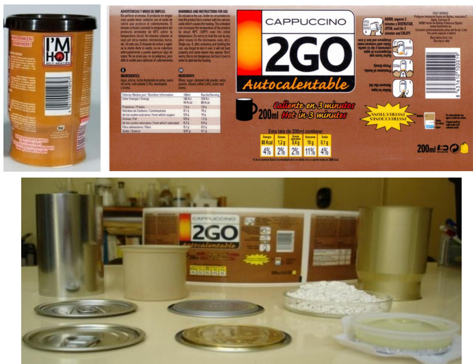
Figure 1.5. Can, label and different components for the commercially available self-heating beverage described in the text.
