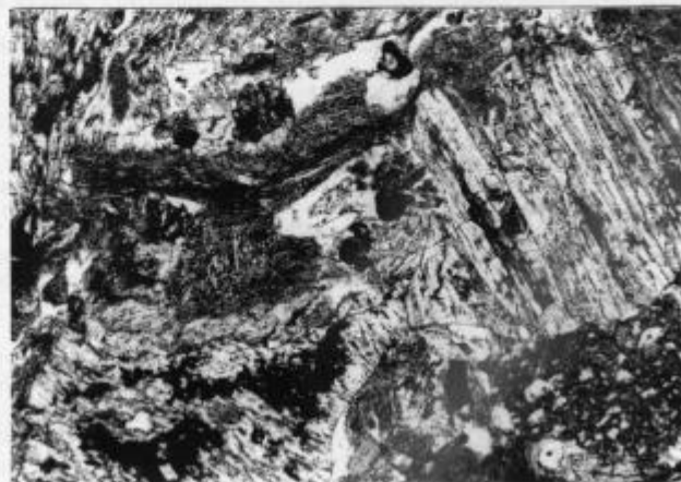
Fig. 3. Resedimented(?) pumice-rich tuff; southern slopes of Krnes. Volcanic glass of a tube pumice is replaced by heulandite, quartz and smectite. Plane polarised light, magnification 14.5 ×
