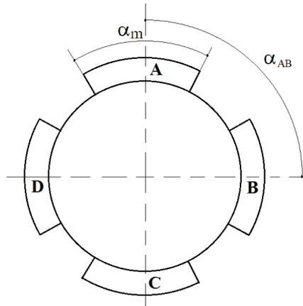
Figure 2: The width ( $\alpha_m$ ) and the relative position ( $\alpha_{AM}$ ) of the magnets
