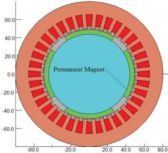
**Figure 1:** Cross-section of synchronous surface-mounted PM generator
