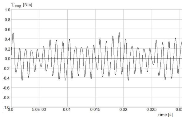
**Figure 5: FEM simulated cogging torque waveform (case 1, Table 1)**
