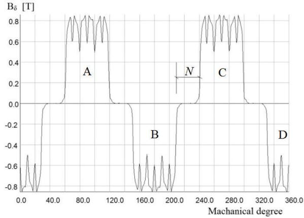
**Figure 3:** Air-gap flux density distribution due to rotor magnets
