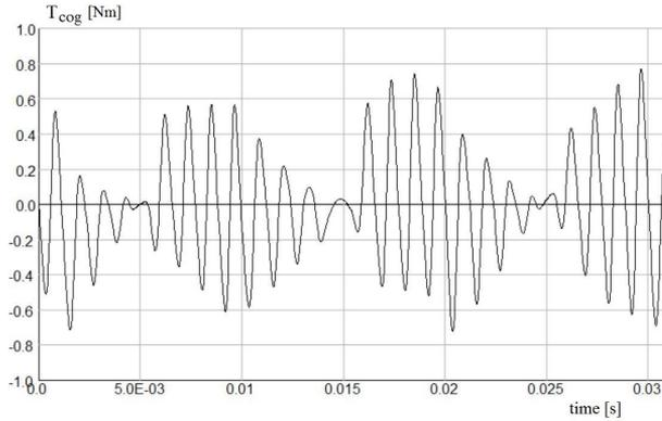
**Figure 6:** FEM simulated cogging torque waveform (case2, Table 1)
