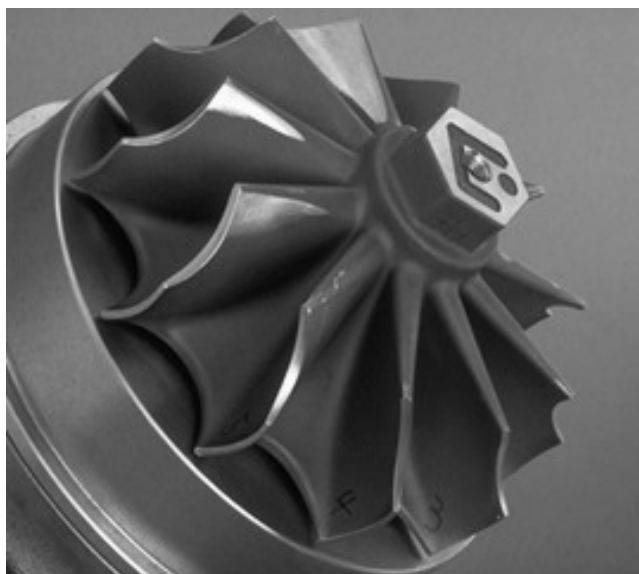
Sl. 1. Gonilnik turbopuhala z 11 lopaticami Fig. 1. Turbocharger impeller with 11 blades
