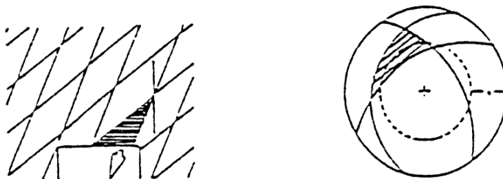
Figure 1b. Conditions leading to rock wedge sliding [5] Slika 1b. Pogoji pri drsenju klina [5]
