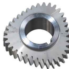
Fig. 7. 3 rd order elliptic helical gear, hobbled
