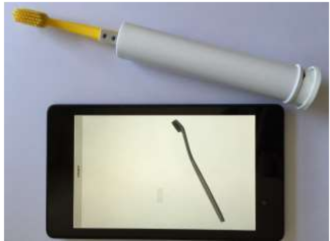
Fig 2 Smart toothbrush prototype with the mobile application
