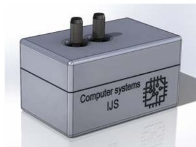
Figure 6: 3D model of the housing, which was printed using 3D printer and PLA plastic material
