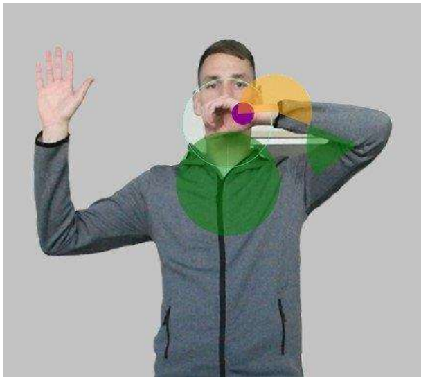
Fig 4 The Kinect application (palm distance from the mouth - violet dot (full circle) means that the palm is positioned correctly in front of the head; the position of the palms in front of the mouth - a light green circle surrounding the mouth indicates the area in which the palm needs to be positioned (the violet dot must be within this circle); position of the wrist in front of the mouth - yellow section of the circle marks the right position of the wrist; the position of the arm - the green section of the circle indicates the right hand position; the position of the head and body; - a green circle section indicates the right position of the head and body)
