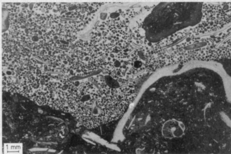
Fig. 14. Passage of biomicrotic limestone into sparitic limestone full of rounded fragments (bioclasts), ooids and intraclasts. Podpeč
