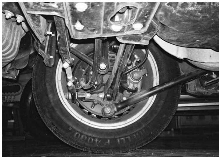
Sl. 13. Zadnja obesa vozila Renault safrane 2.2 RT Fig. 13. Back suspension of the Renault Safrane 2.2 RT
