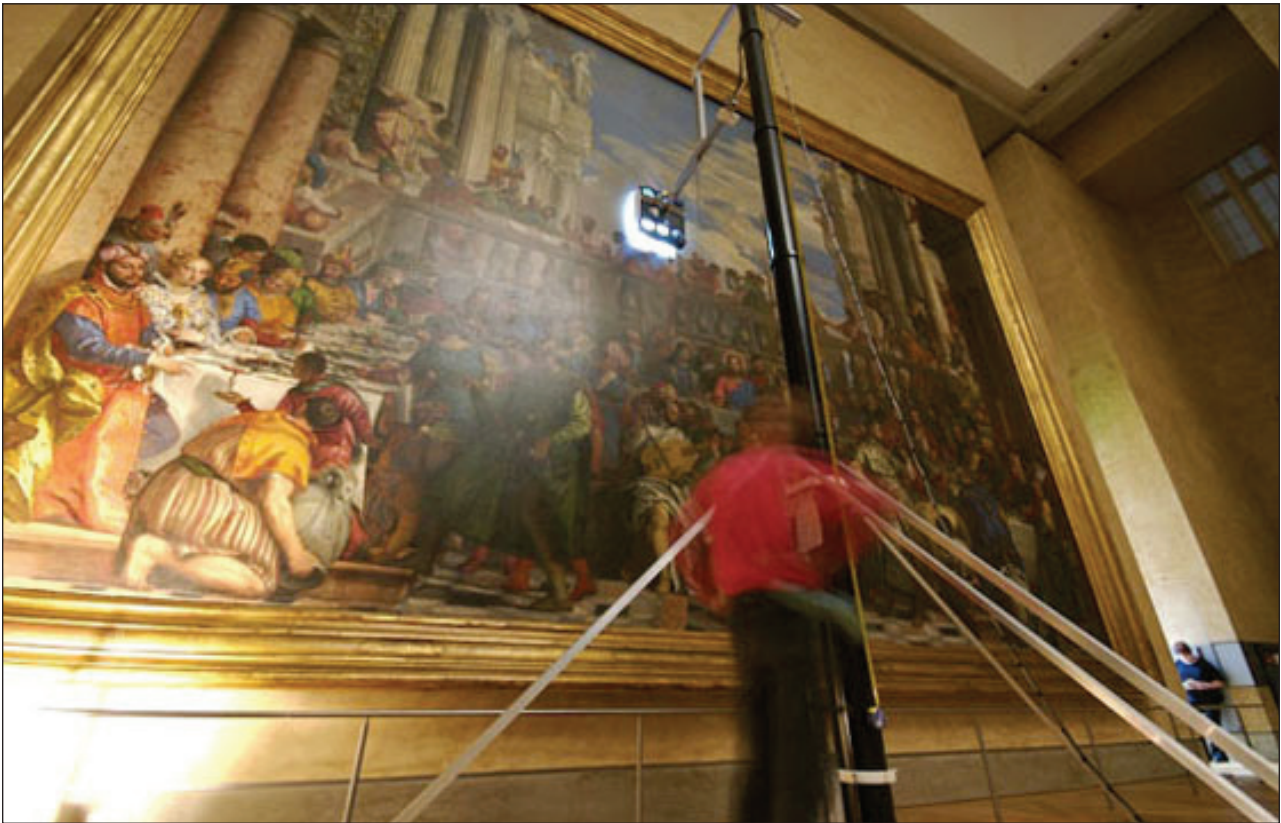
Figure 4: The specially-built scanner and rig used for scanning Paolo Veronese's Nozze di Cana (Source: © Factum Arte).
