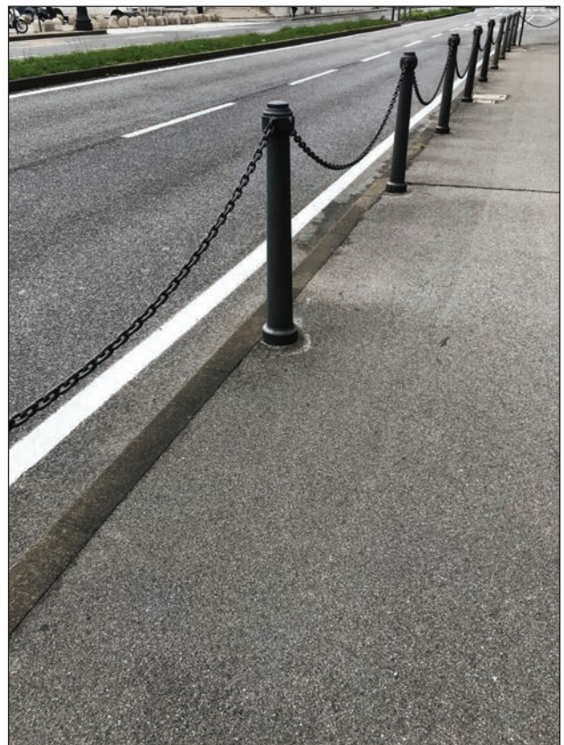
Figure 12: Urban furnishing (bollard chain) as barrier, when its presence cannot be checked by the white stick. Corso Cavour, Trieste, 2018 (Photo: G. A.).
