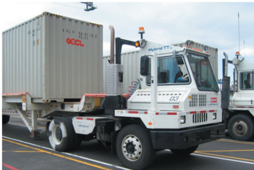
Fig. 2. Utility tractor rig
