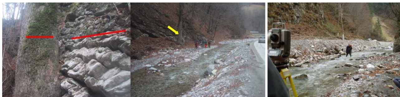
Figure 2: Post flood survey: a) Examples of a high water mark. The vegetation removed from the rocky bank and the moss drenched with silt on the downstream side of the tree show the highest level reached by floodwater (red line). b) The arrow shows a tree with the flood mark and a phase of the topographic survey of the river section. c) Surveying the stream bed.
